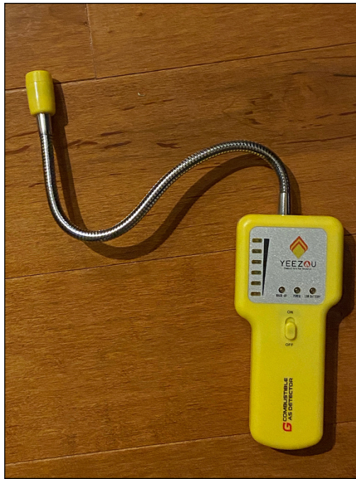
FIGURE 16-9: A handheld leak detector is a safe, dependable way to check pipes, hoses, and appliances for a propane leak.
