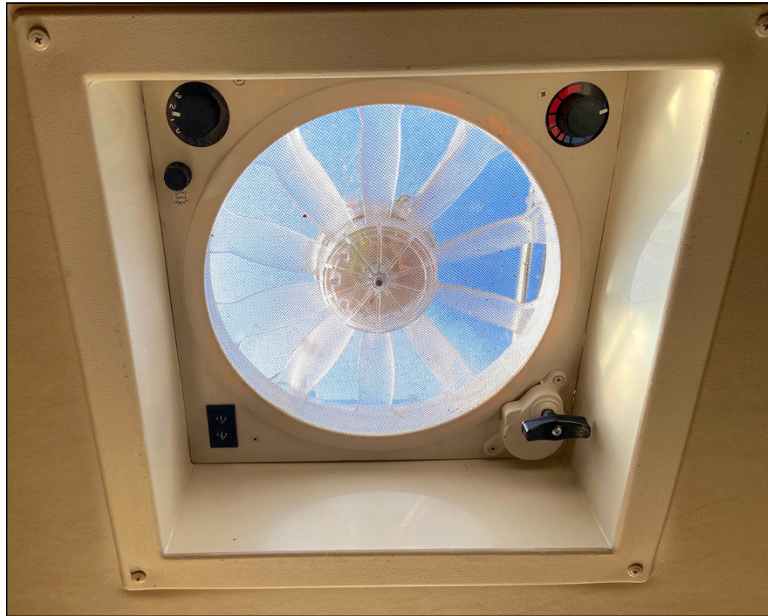
FIGURE 17-1: A typical rooftop ventilating fan can help cool down an RV when combined with a couple of open windows.
