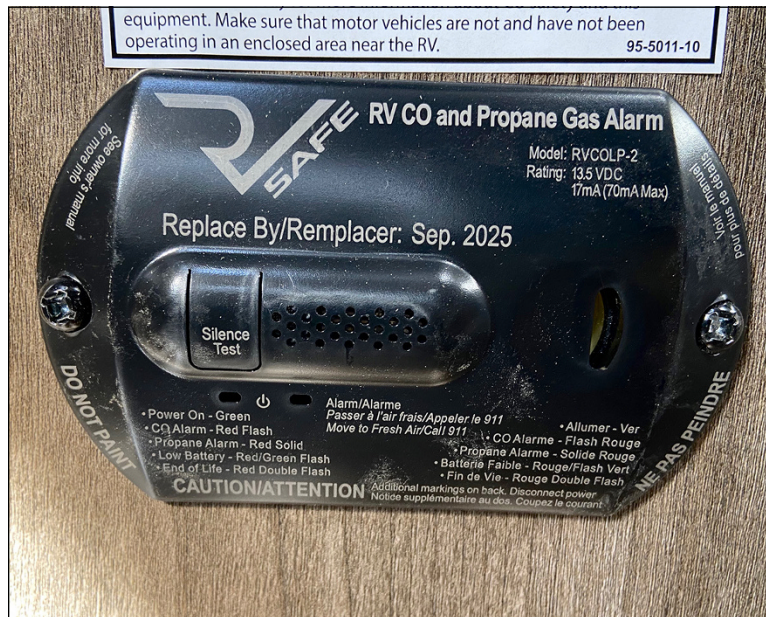
FIGURE 16-8: A combination carbon monoxide and propane leak detector alarm.
