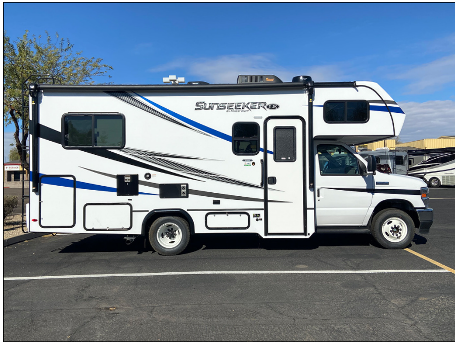
FIGURE 2-4: Class C motorhomes have a distinctive hump over the truck cab.
