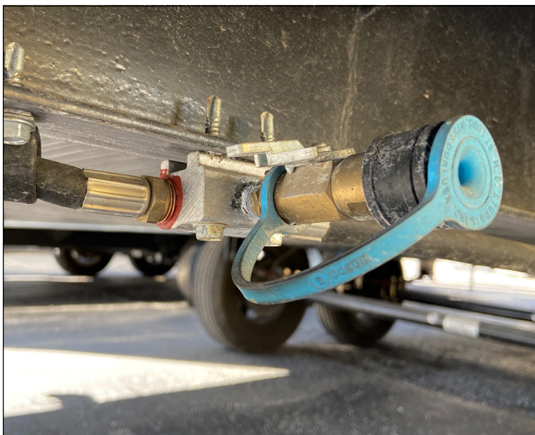
FIGURE 16-1: Your trailer or motorhome may have one or more outdoor propane outlets to let you use your rig's gas supply for your grill and more.
