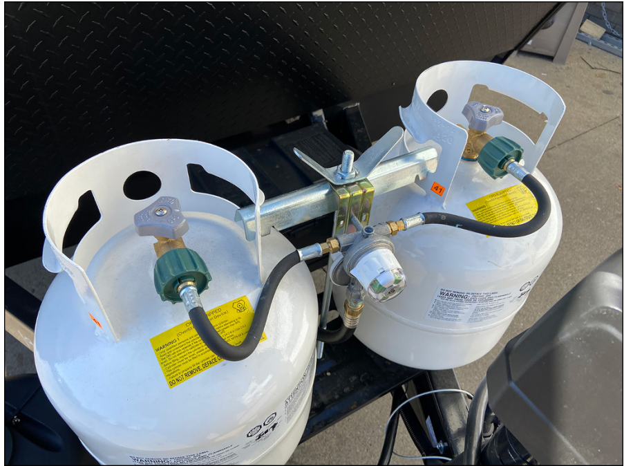
FIGURE 16-2: Portable, refillable propane tanks on a trailer are typically mounted vertically up front on the trailer's A-frame.
