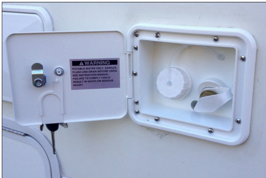
FIGURE 15-2: The freshwater holding tank inlet.
