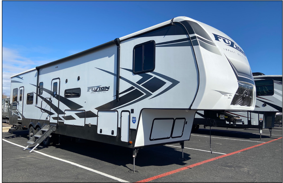
FIGURE 2-10: The distinctive overhanging design of a fifth-wheel trailer requires a special kind of hitch mounted in the bed of a pickup truck or other utility truck.
