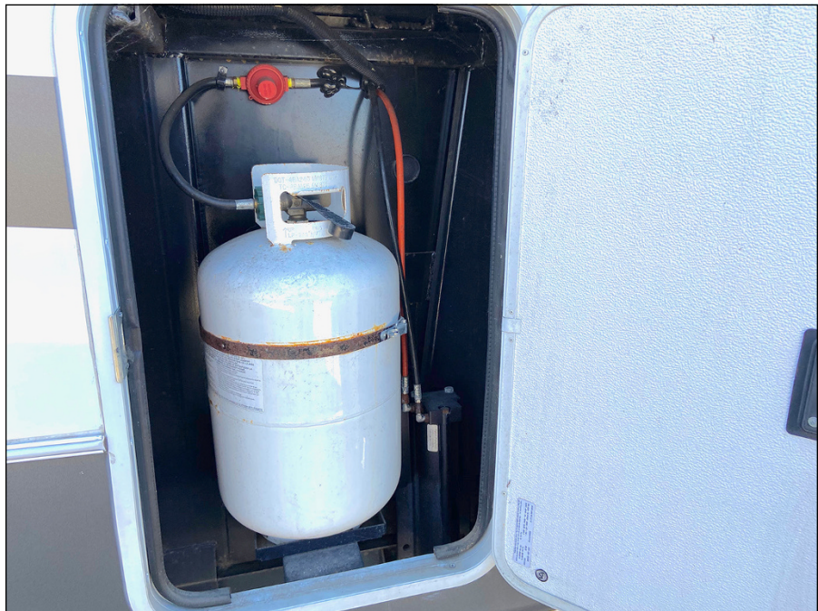
FIGURE 16-3: Propane tanks on large trailers and fifth wheels may sometimes be inside a cabinet or pull-out drawer.
