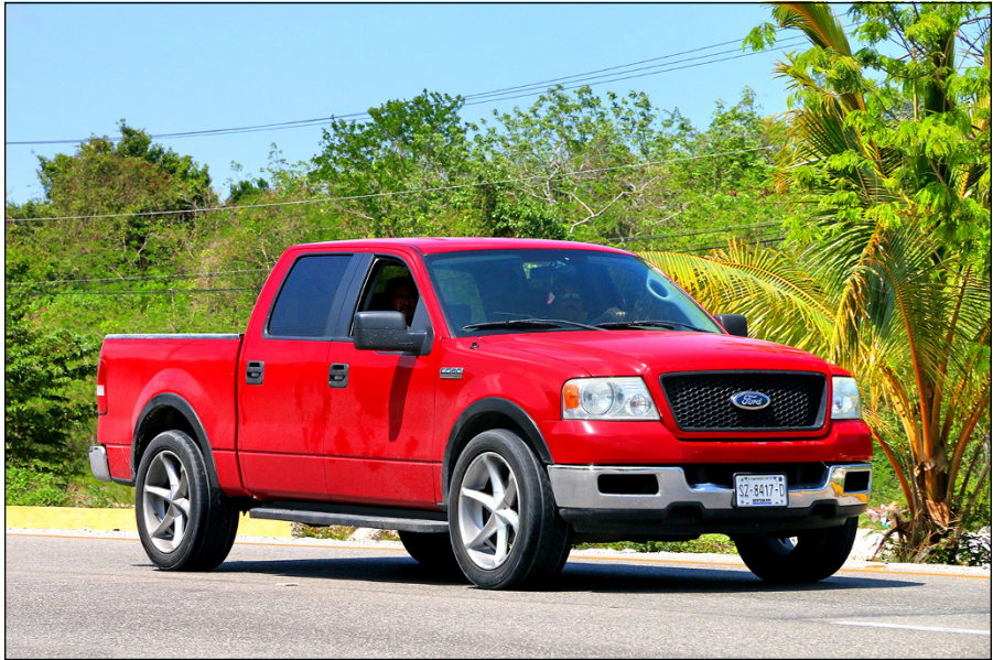
FIGURE 7-1: Ford F-150 crew cab with two rows of seats and four full-size doors. Crew cabs have the most interior space and can seat up to five adults.
