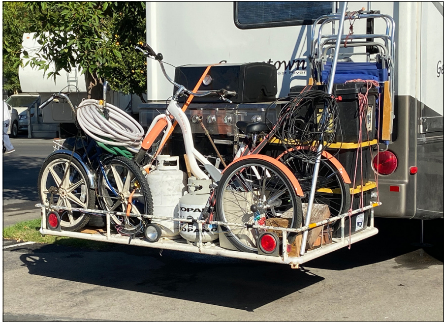
FIGURE 8-1: Just because it fits doesn't make it safe. Most weight-carrying receivers on the backs of trailers aren't designed to safely support more than 200 to 300 pounds.
