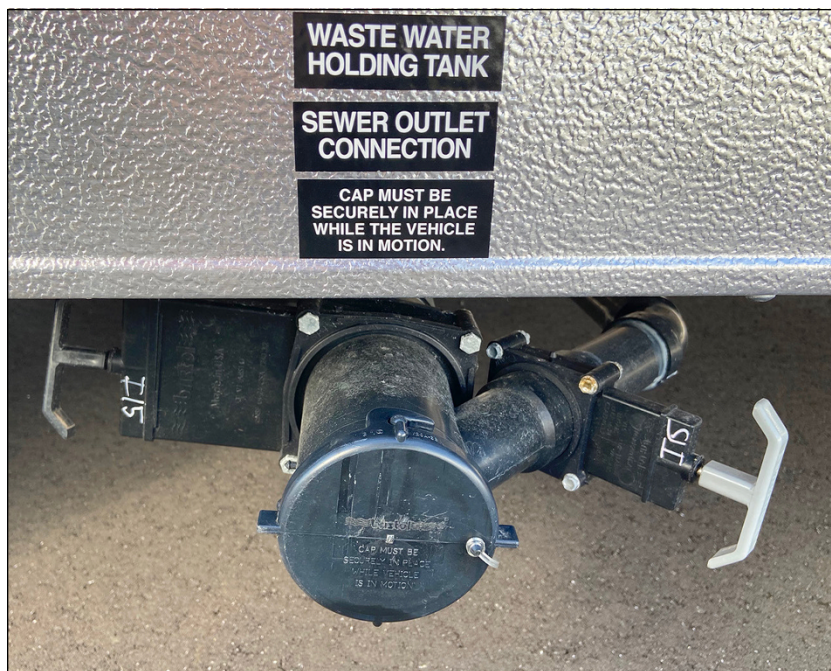
FIGURE 15-6: A typical sewer (wastewater) drain valve has a 3-inch pipe where your waste drains out, a graywater handle, and a blackwater handle.
