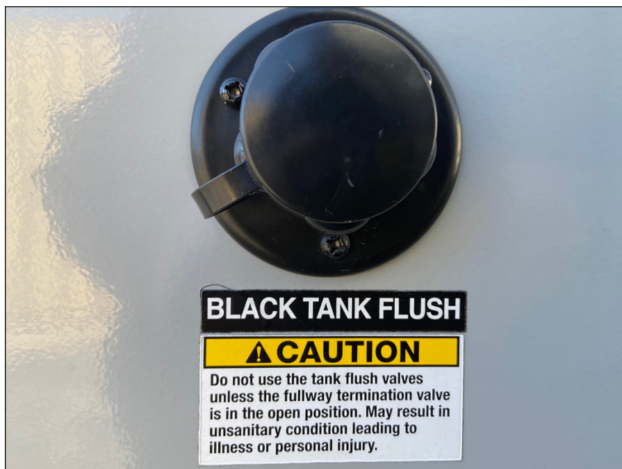
FIGURE 15-9: Your rig may have a blackwater tank rinse-out flush valve. Don’t get it confused with your city water inlet!
