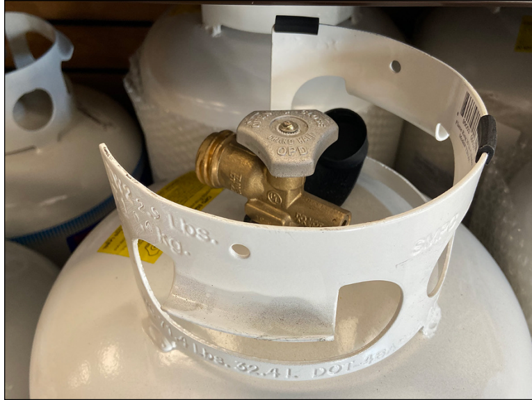
FIGURE 16-4: The collar of a portable, refillable DOT propane tank contains lots of information.
