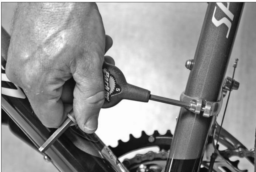
Figure 14-12: Removing the pivot bolt.
