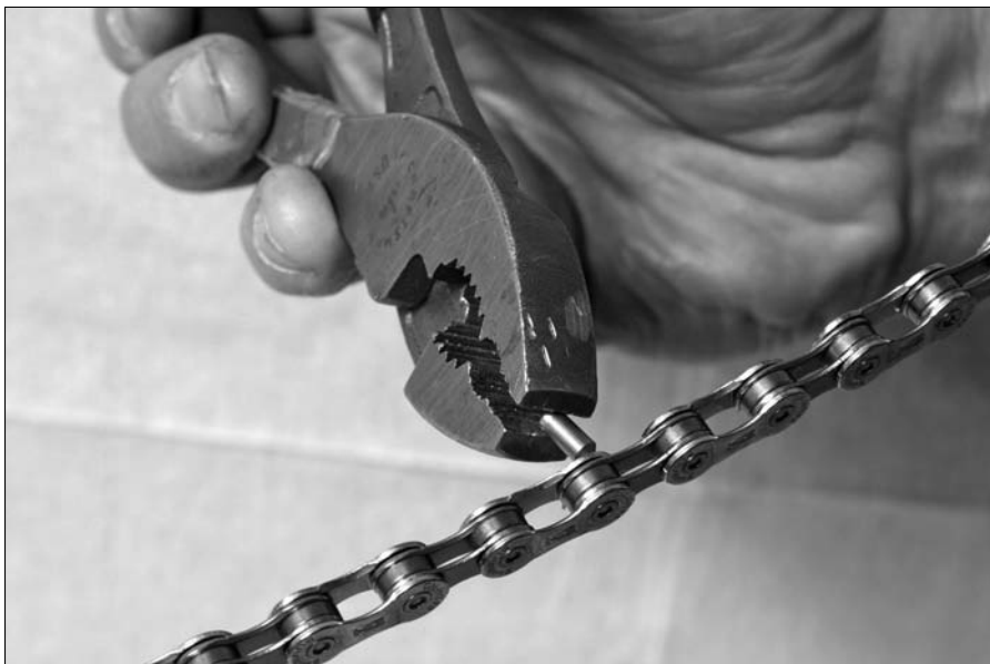
Figure 10-15: Snapping off the replacement pin's head.
