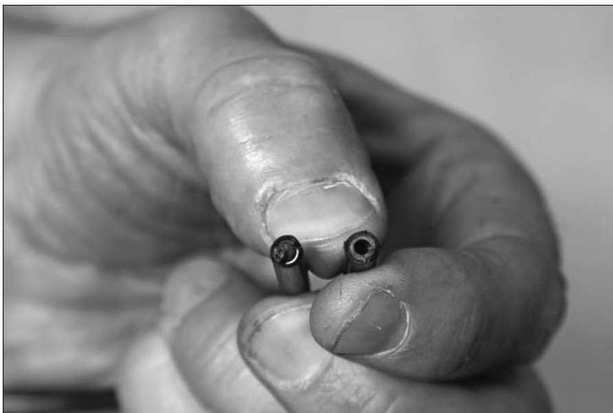
Figure 8-22: Properly cut cable housing.
