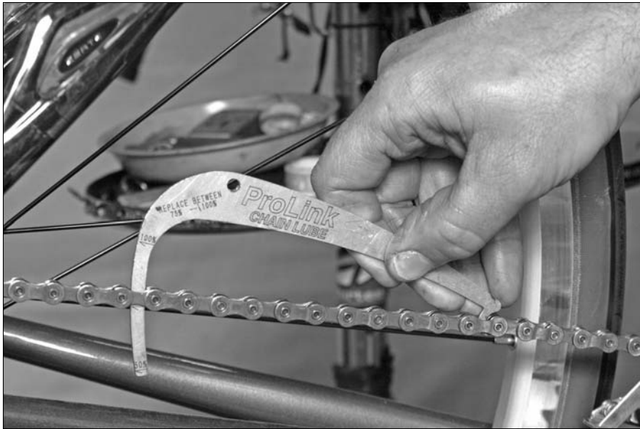
Figure 10-7: A chain measuring tool makes measuring a chain easy.
