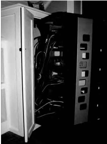
Figure 2-3: Danny's rack allows access to his back panels without disconnect- ing wires.
