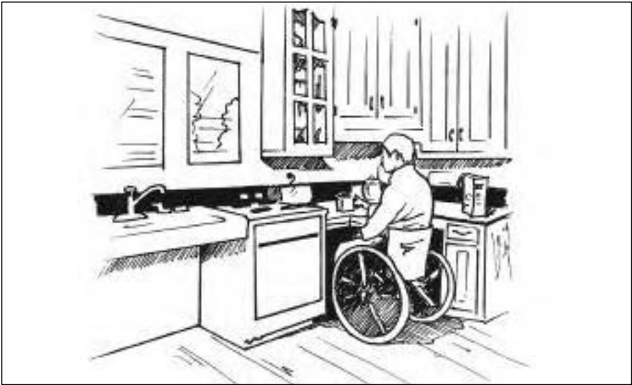
FIGURE 4.3— Accessible design calls for wider doors, a way to get into the house without stairs, key services on the first floor, and sinks that can be used by someone in a wheelchair.
