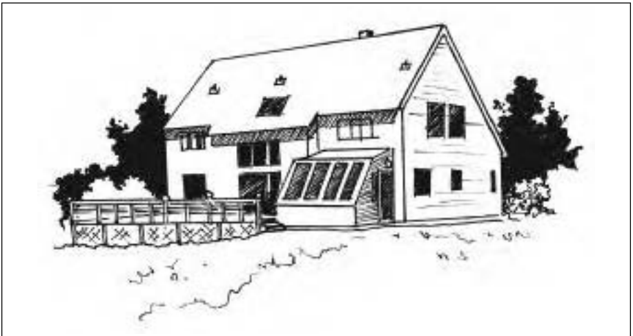
FIGURE 4.5— To optimize passive solar heating, the longer axis of the house should be oriented east-west, providing more area for south-facing windows.
