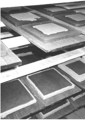
Figure 2.30 Slip coated encaustic tiles left to dry.
