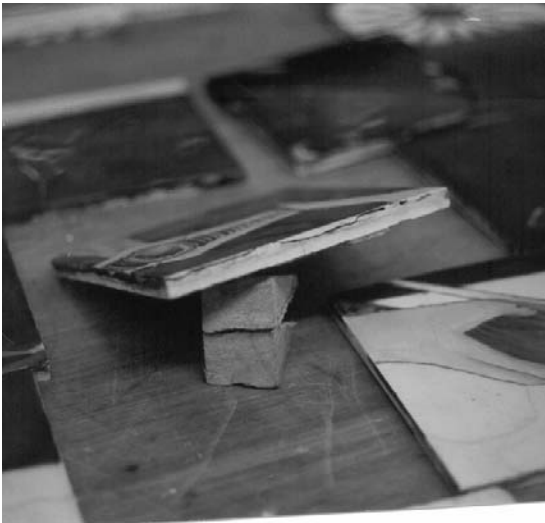
Figure 5.22 Delamination due to frost action.
