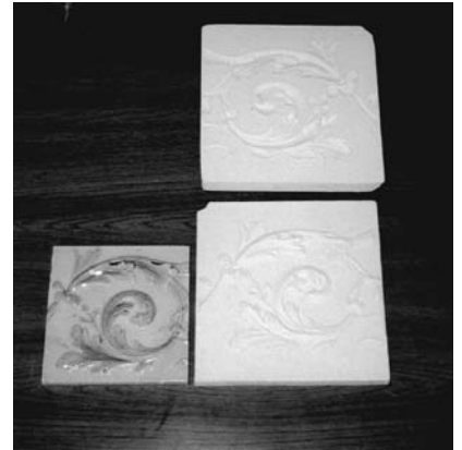
Figure 2.29 Tiles and mould together showing allowance for shrinkage.
