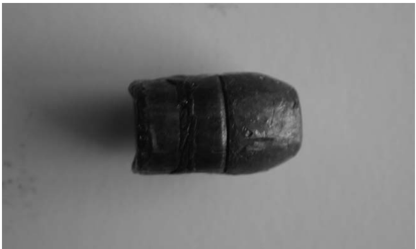
Figure 3.15 Fired bullet with no rifling impressions.
