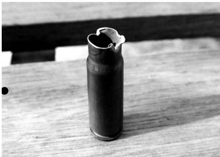
Figure 4.27 Deformed 7.62 \times 39 cartridge case mouth.
