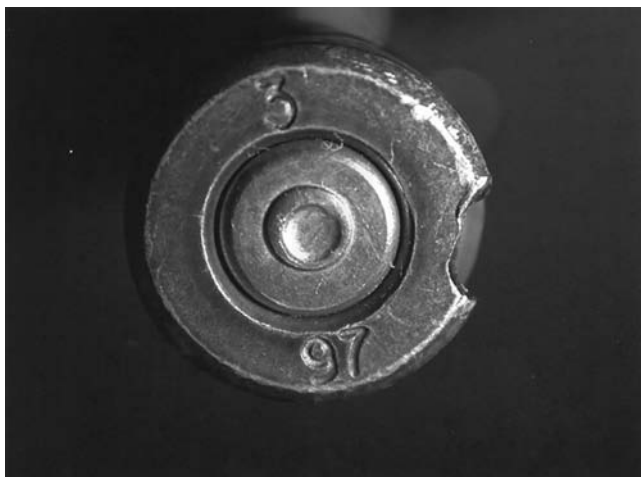
Figure 4.28 Deformed 7.62 × 39 cartridge case head.
