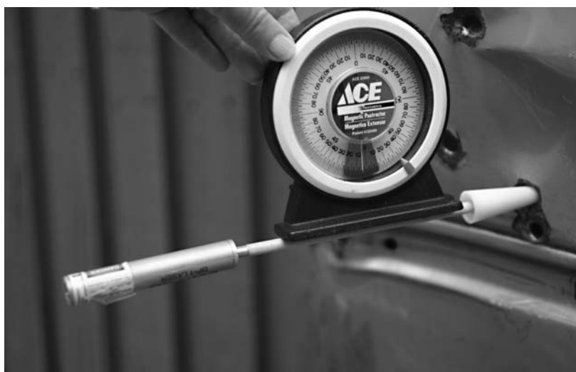
Figure 4.16 Using an angle gauge.
