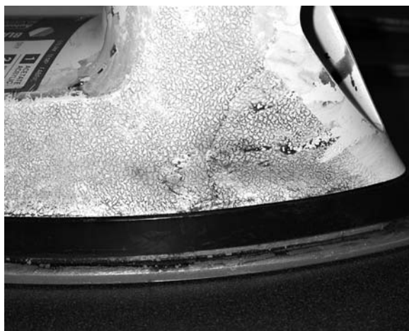
Figure 7.2 Soot on iron.
