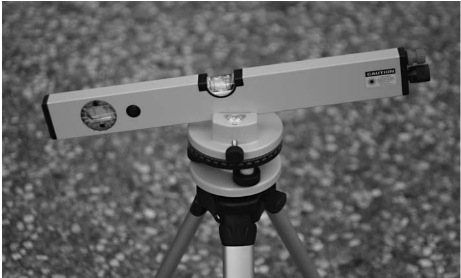
Figure 4.24 Laser level modified for vertical rotation.
