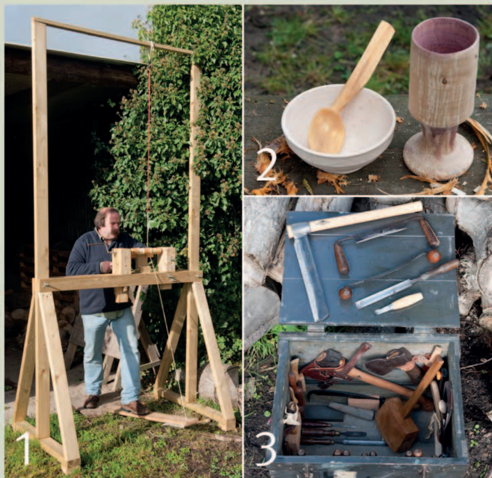
1. A traditional pole lathe doesn't need an electrical power supply and can be set up anywhere, even in the woods. 2. A pine bowl and green wood goblet turned on a pole lathe, with a hand-carved cherrywood spoon. 3. Green woodworking tools , including a froe (top left) for splitting wood and various sharp knives.
