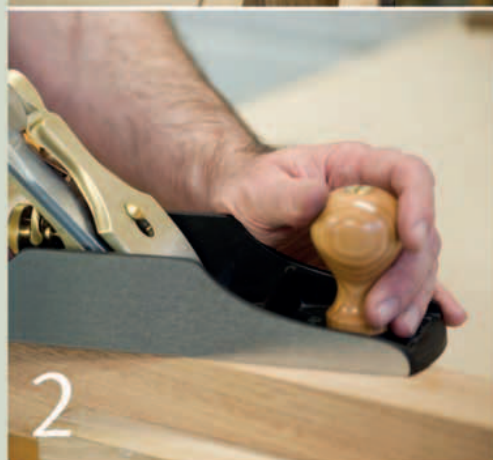
1. Use your thumb knuckle to align a saw as you start to cut. 2. A bench plane smooths rough surfaces. Check your progress by laying the plane on its side to see how flat the wood is. 3. A sharp chisel makes neat work of a tenon (see page 277). 4. Mark wood accurately with a steel ruler.
