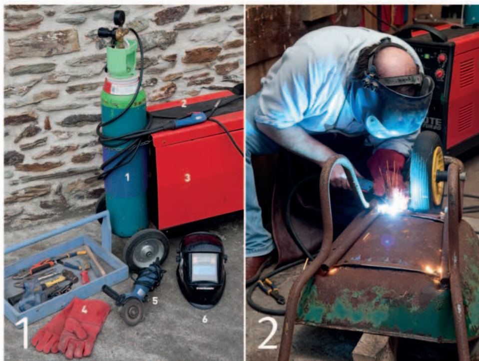
1. The essential MIG welding kit doesn't require a huge number of items. Above left, there is the shield gas (1), welding gun (2), welder power supply (3), heavyweight welding gloves (4), grinder (5), and welding mask (6). 2. Learn the basic skills of welding and they can be put to use surprisingly frequently. This wheelbarrow has been a trusty friend over the years, so when its bottom fell away, a bit of tender loving care with the welder meant that all was well again.
