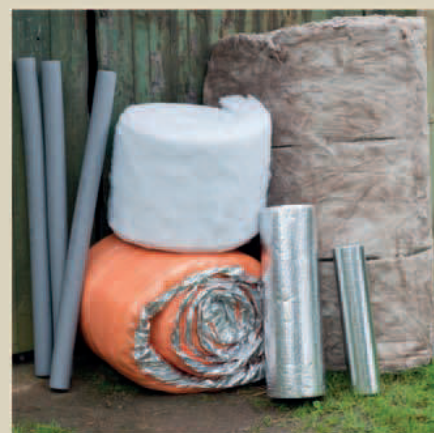
Insulation for every situation From left: expanded foam for pipework, recycled plastic fleece, a jacket for a hot water tank, foil reflectors for radiators, and a large roll of sheep's-wool attic insulation.
