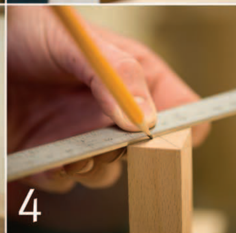
1. Use your thumb knuckle to align a saw as you start to cut. 2. A bench plane smooths rough surfaces. Check your progress by laying the plane on its side to see how flat the wood is. 3. A sharp chisel makes neat work of a tenon (see page 277). 4. Mark wood accurately with a steel ruler.
