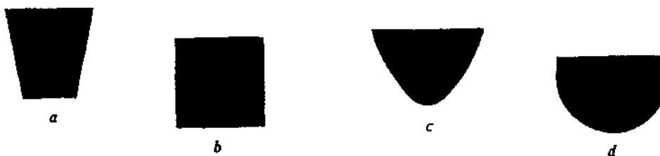
FIG. 27—THE EFFECT OF CONTOUR ON JUDGMENT OF PROPORTIONS Proportions should be judged before reading this caption. Over-all proportions: a and b both 1, c and d both M .
