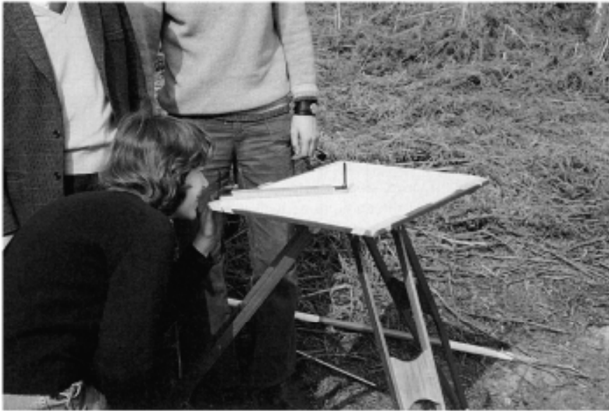
Figure 4.6 Plane table surveying.
