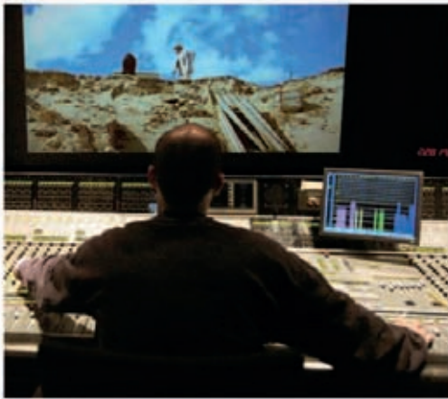
📌 The sound mixing desk is where the various tracks of human dialogue, sound effects, and music are combined to create an original to transfer to the film negative.
