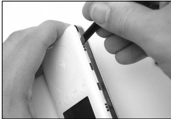
Figure 11.12 Unclip all the Tabs
