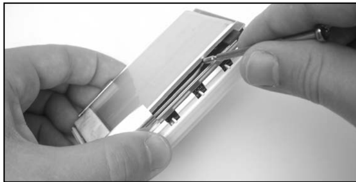
Figure 11.40 Pulling the Battery and Hard Drive Apart
