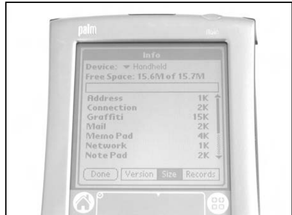
Figure 13.42 After Hack: Palm m505 With 16MB RAM
