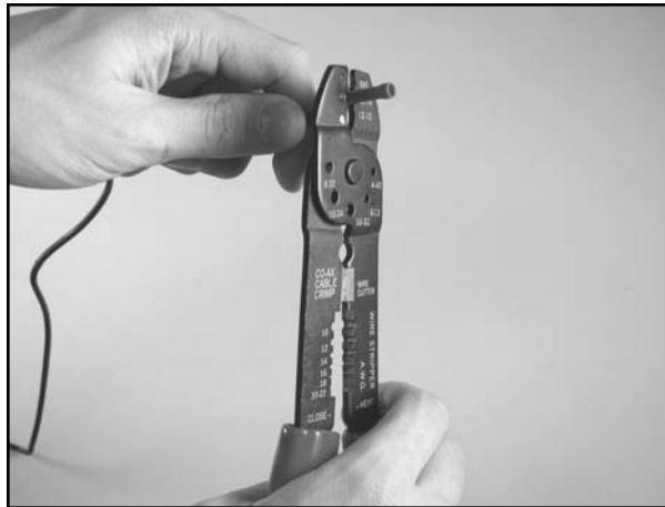
Figure 5.47 Crimping the Wire
