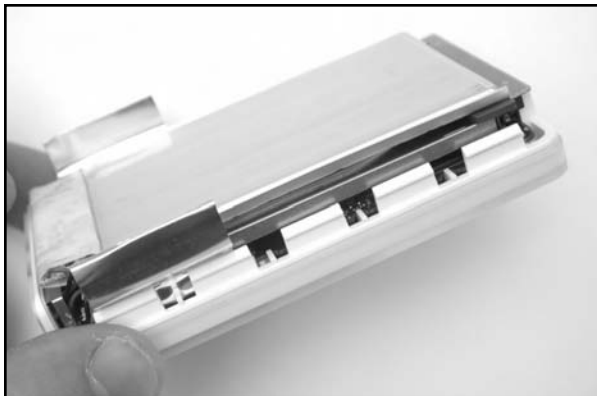
Figure 11.52 Battery Back in Place
