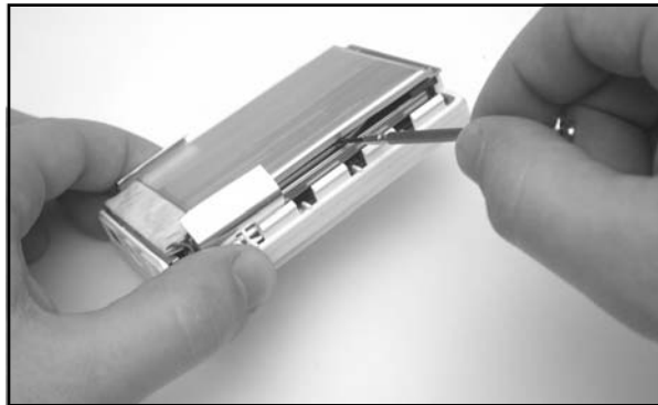
Figure 11.18 Prying the Battery from the Rubber Strips
