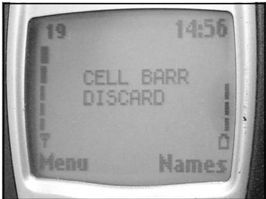
Figure 12.31 Test 19: Ignoring Barred Base Stations
