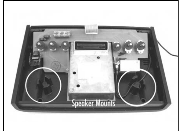
Figure 7.23 Receptacles Inside the Case for Speakers
