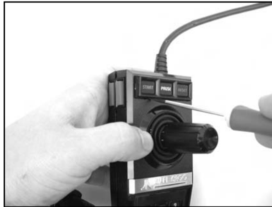
Figure 8.21 Removing the Upper Bezel
