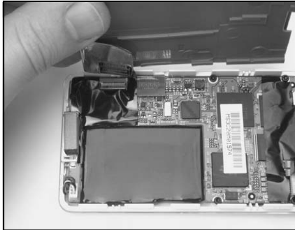
Figure 11.33 Reattaching the Hard Drive
