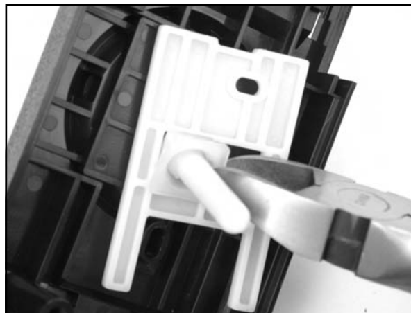
Figure 8.26 Freeing the Joystick
