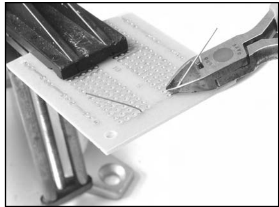
Figure 2.31 Snipping Off the Remaining Component Lead
