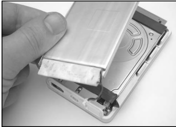
Figure 11.19 Removing the Old Battery
