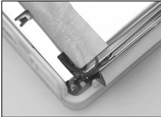
Figure 11.22 Power Cable Safely Tucked Away
