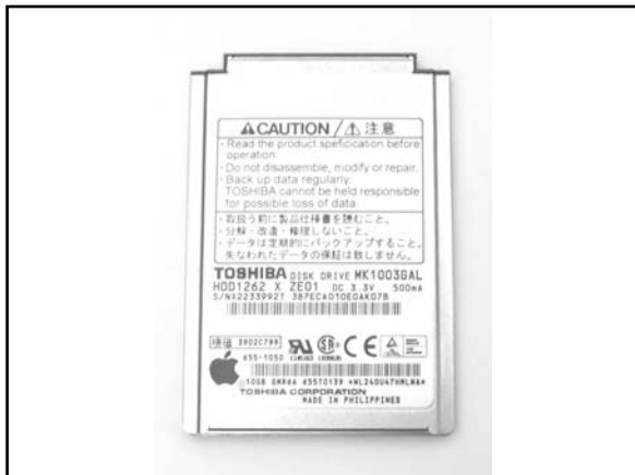
Figure 11.37 A 10GB iPod Hard Drive
