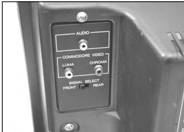
Figure 8.71 Commodore 1702 Rear Input Jacks
