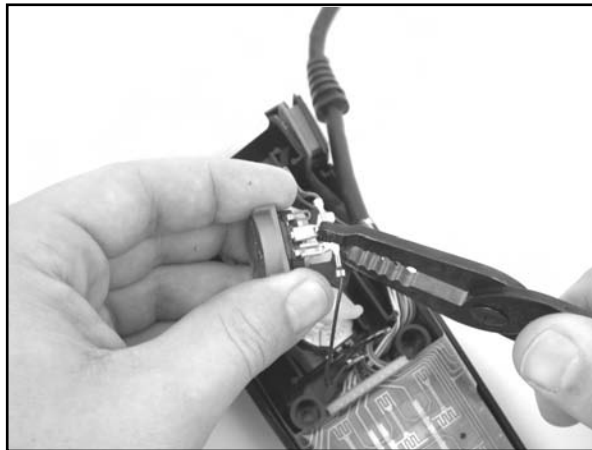
Figure 8.24 Removing Wires from the Upper 5200 Pot
