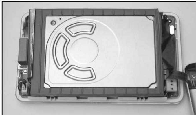
Figure 11.34 Hard Drive Back in Place
