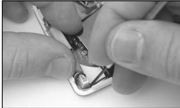
Figure 11.31 Tucking In the Power Cable
