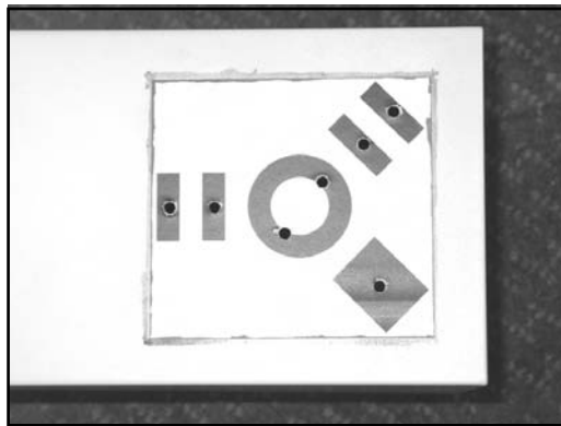
Figure 4.13 Template With Pilot Holes and Initial Cuts
