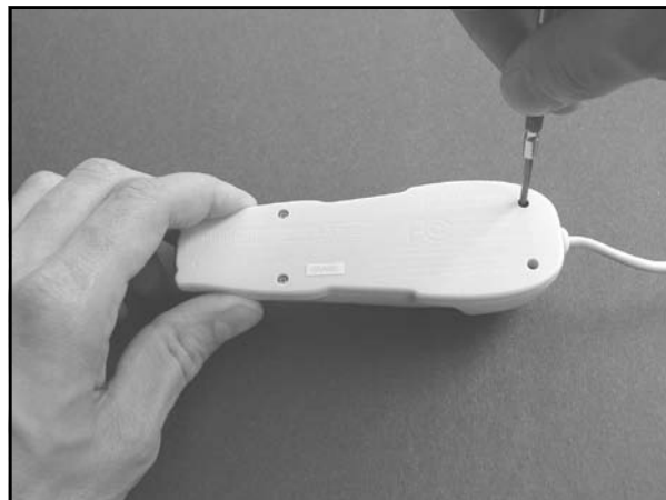
Figure 3.4 Unscrewing the CueCat
