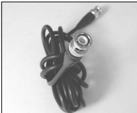
Figure 10.4 An Unmodified Thinnet Cable
