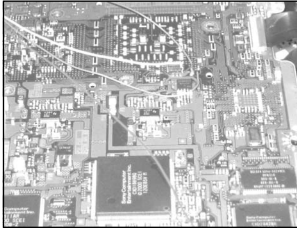
Figure 9.12 Installed SIO Wiring
