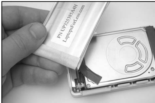
Figure 11.20 Connecting the New Battery
