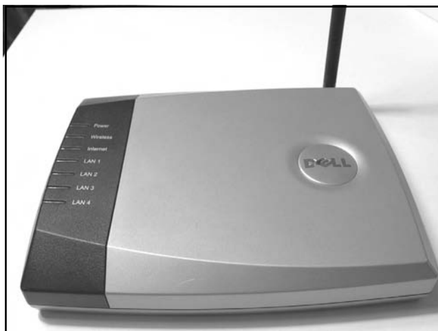
Figure 10.17 A Dell 1184 Access Point
