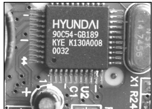
Figure 3.34 Hack Complete: Pin 10 of Microprocessor Lifted (Close-Up)
