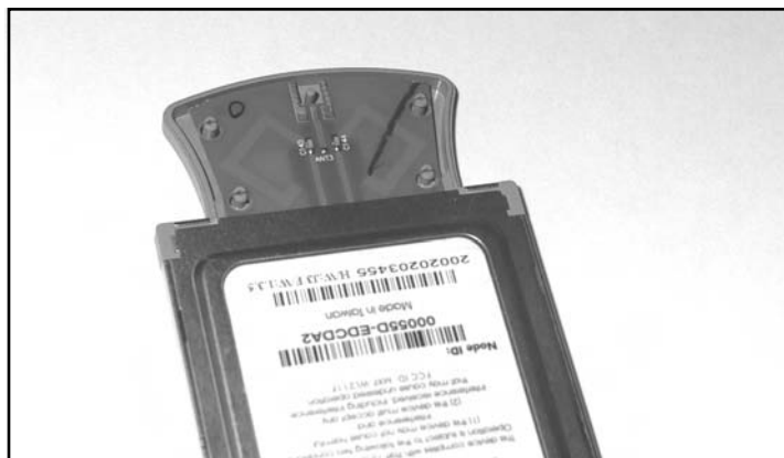
Figure 10.7 Inside the Antenna Compartment
