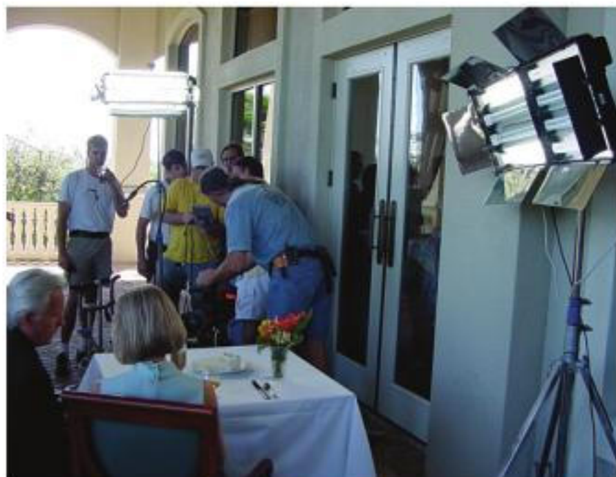
FIGURE 2.14 Pampa lights with daylight-balance bulbs in use on an open-shade day exterior. A four-bank unit keys them from the side, and a two-bank unit over the camera gives a soft fill. (Photos courtesy of Owen Stephens, Pampa Light.)
