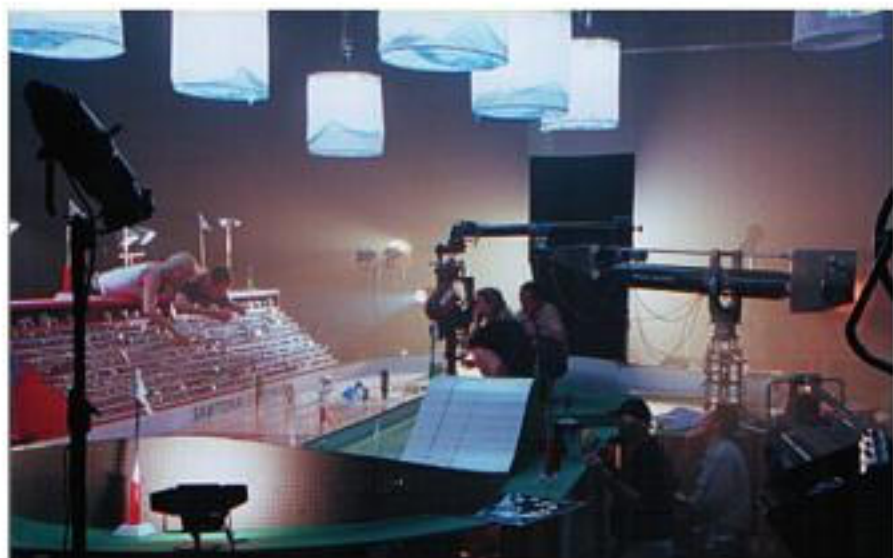
FIGURE 12.3 Spacelights create an ambient base for a snorkle rig shot; some Source Four lekos add the highlights. Macro and snorkle shots almost always require a high f /stop and thus must be lit to a fairly high level. (Photo courtesy of Mark Weingartner.)
