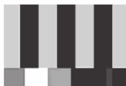
FIGURE 5.7 Blue-only color bars—notice that the bands are of equal intensity and in the upper portion the large and small bars are equally gray or black.
