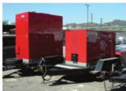
FIGURE 8.3 Two sizes of AC generators, both of them “tow-away,” meaning they are towed.
