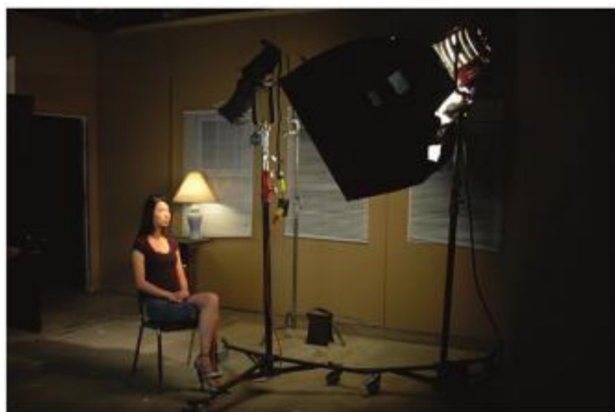
FIGURE 3.13 Behind-the-scenes for the hard light vs. soft light test. A Source Four leko is used for hard light. For the soft light, a 2K with a Chimera softbox is used. A bleached muslin 4' × 4' was added for the softest light.
