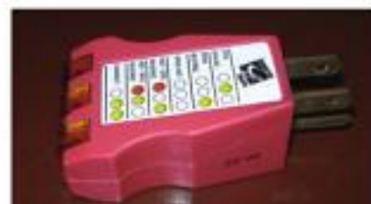
FIGURE 8.14 A circuit tester is important not only for safety, it is also a quick way to check if a line is hot or not.
