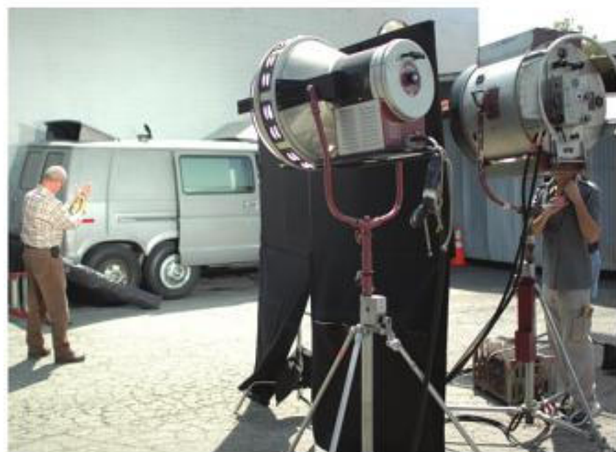
FIGURE 2.5 A side-by-side comparison of a Brute Arc (on the right) and a 12K HMI PAR. Both units are mounted on Mole Litewater crank-up stands.
