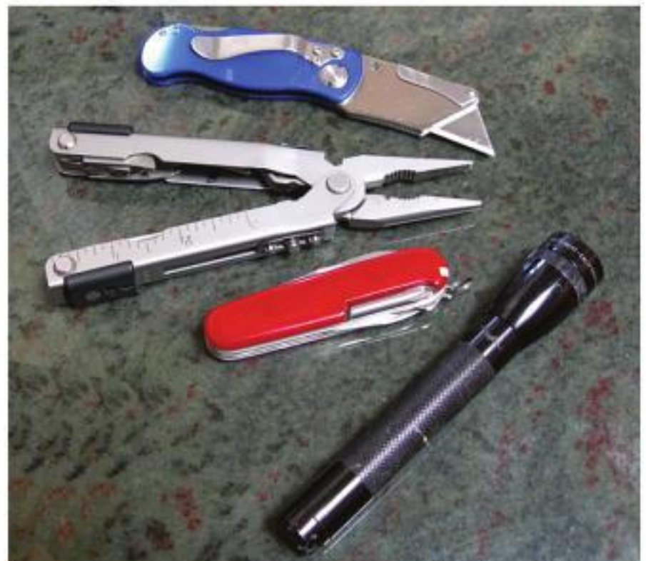
FIGURE 10.5 The basics that every technician should have on the set: a cutter, some kind of multi-tool, a Swiss Army knife, and a flashlight. One additional essential for grips and electricians: work gloves.
