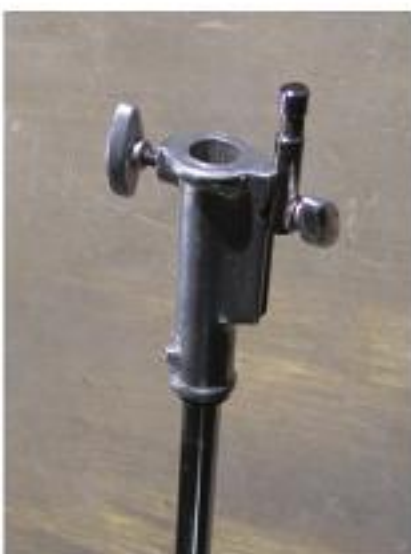
FIGURE 9.1 A combo head with both \frac{5}{8} " baby stud and a 1\frac{1}{8} " junior receiver.
