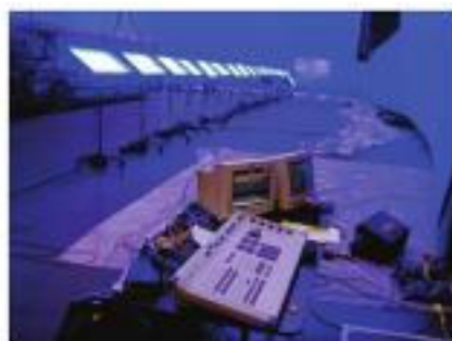
FIGURE 12.2 A dimmer system controls Kino Flo units for a large blue screen shot. (Photo courtesy of Kino Flo, Inc.)
