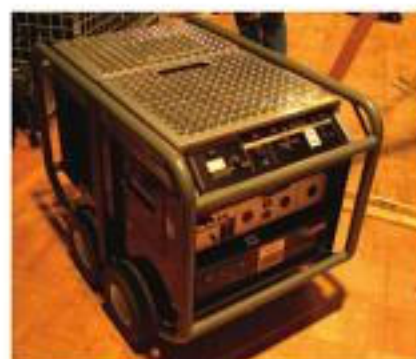
FIGURE 8.4 Small portable sources are known as “putt-putt” generators, usually about 5500 watts. Those that are adapted for film usually have crystal sync, thus making them suitable for use with HMI lights.
