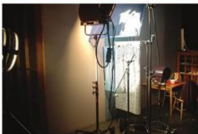
FIGURE 3.20 Adding texture to lights. Charlie bars (vertical bars, in this case made from tape on an open frame) and also some lace create texture in the scene. A Mole beam projector is the key; a 4K soft through some light blue gel ( \frac{1}{4} CTB or Color Temperature Blue) simulates skylight, while the beam projector recreates direct sun.
