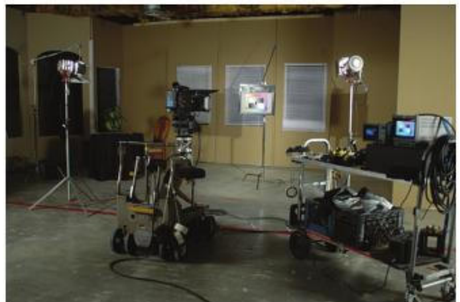
FIGURE 5.8 A typical setup for the test chart. In this case, two Tweenies at a 45° angle are at exactly the same distance and angle from the Chroma du Monde chart for even lighting. Each Tweenie has a double scrim in it to reduce the light. This is for setting backfocus, which requires that the lens be as wide open as possible.
