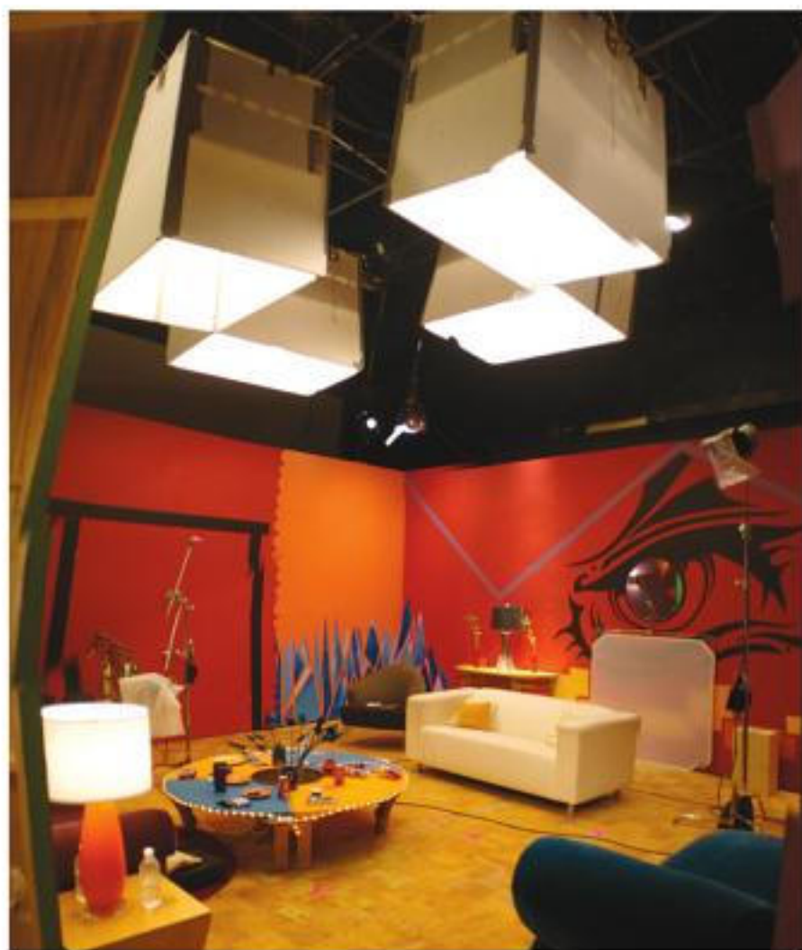
FIGURE 4.16 Reality show set (a) and the set-built softboxes (b) and (c) that provide the overall ambient light.
