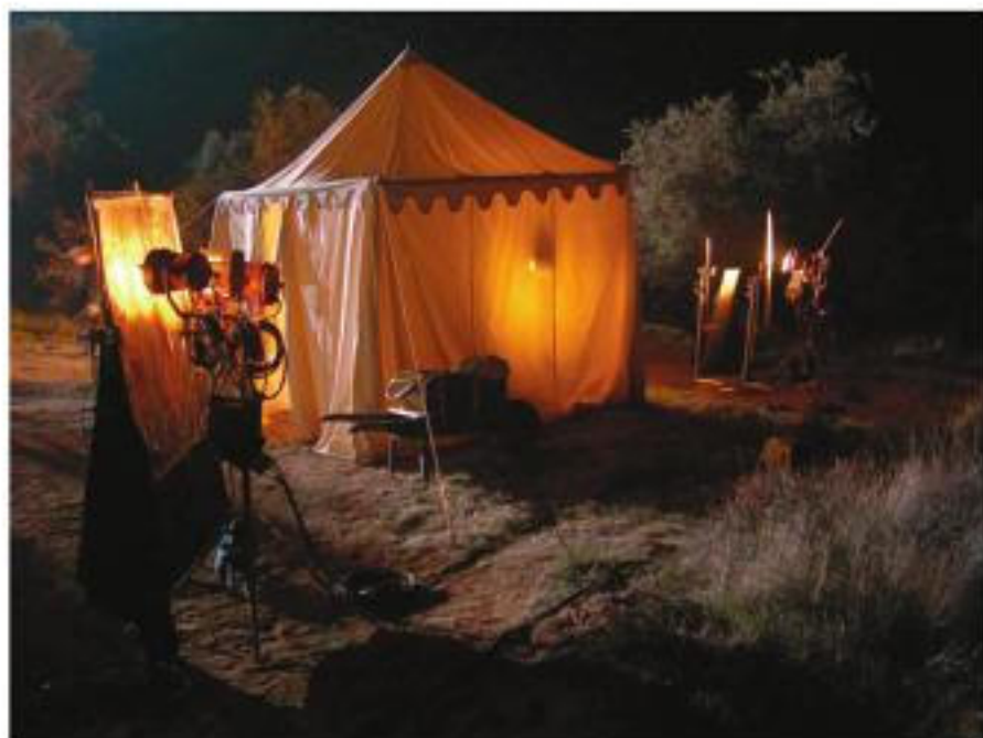
FIGURE 4.3 The fire effect was provided by three fire rigs. These are a Mighty Mole, a Baby-Baby, and a Mickie Mole on a triple header with all lights run through a three-channel flickerbox. See Figure 4.4 for a closeup of the fire rig.
