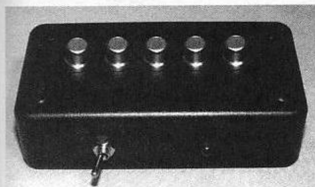
Figure 5-10 The multiple camera auto switcher completed.
