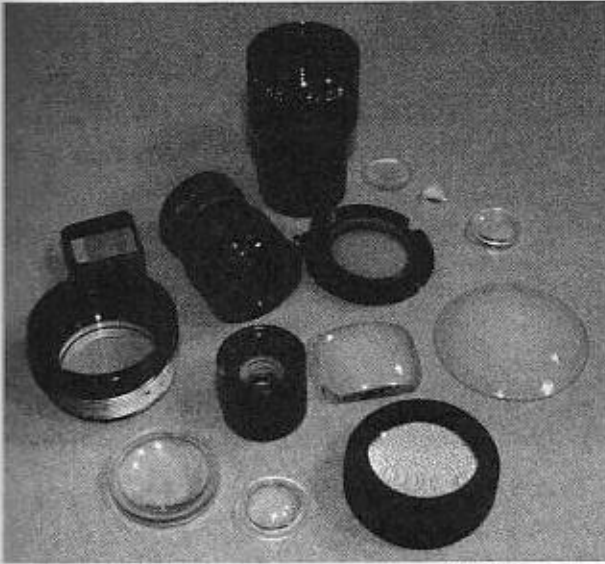
Figure 8-17 An assortment of lenses used for laser focusing tests.
