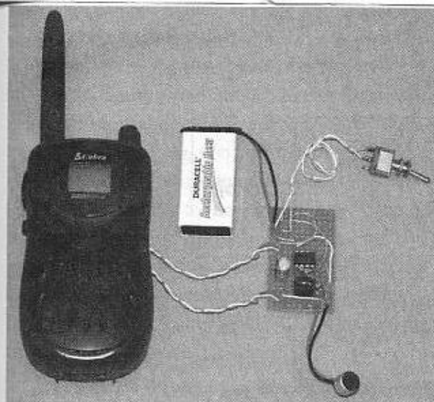
Figure 9-7 Modified radio showing microphone and transmit button extension wires.
