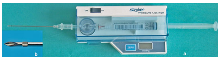
FIGURE 14.1 (a) Intra-compartmental pressure monitor, (b) needle with side port for compartment pressure monitoring
