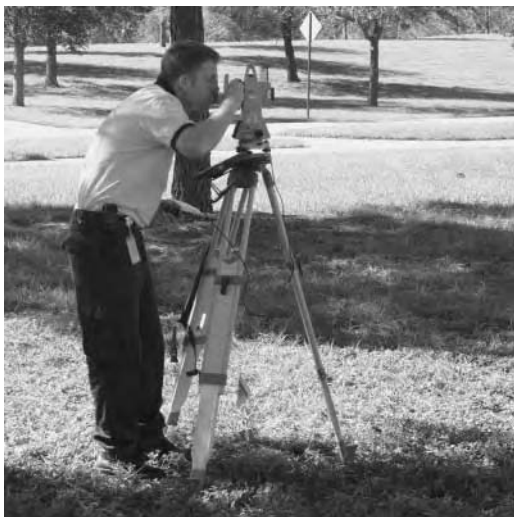
Figure 6.3 Orange County Crime Scene investigator Ronnie Murdock using a total station transit. (Photo courtesy of J. Mulligan.)
