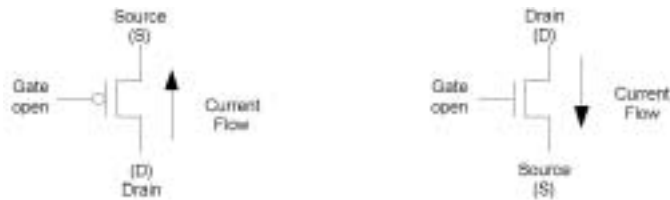
Figure 2.2 PMOS gate open and NMOS gate open.
