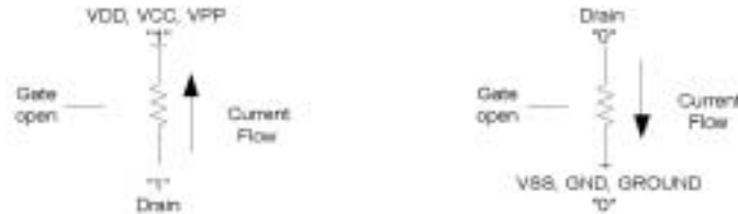
Figure 2.4 PMOS generating a "1" and NMOS generating a "0."
