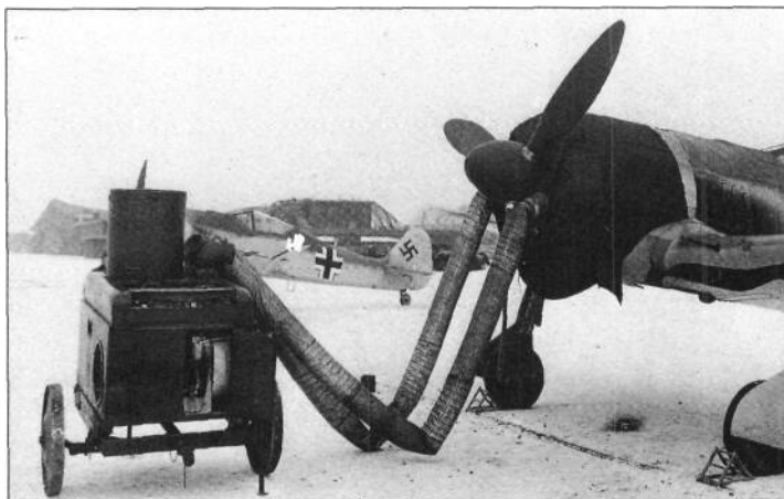
Above and right What the well-dressed Fw 190F wore in the depths of winter. Heating trollies and tents were available only for the lucky few! The latter were often reserved for aircraft undergoing in-the-field maintenance, as conditions often proved too bitter in the depths of winter for 'black men' to work outdoors for any period of time. Note that 'White N' has had a toned down cross applied to its fuselage, although its overall effect is spoiled somewhat by the full-colour Staffel markings
