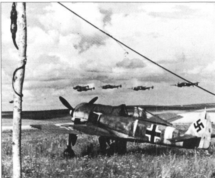
Seen in Rumania in July 1944, a I.Gruppe Schlacht Fw 190 sits quietly in the high grass as an impressive formation of five Bf 110s cruises past at low level. Note the tropical filter fitted to the F-8, which helped keep the sand and dust of the dry plains out of the BMW during taxiing and take-off
