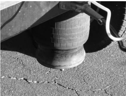
Figure 19.39 Air bags to raise or lower trailer.
