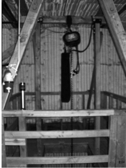
Figure 19.82 Rigging a chain motor rigged for lifting to the perms.
