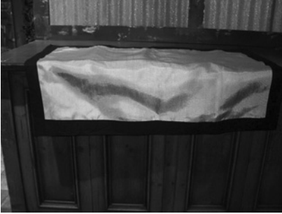
Figure 19.138 Refro seal cloth (fire-retarding/proof cloth).
