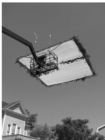
Figure 19.156 Fly swatter with plastic ivy (breaks up the frame edge).
