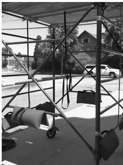
Figure 19.153 How to safety tie down a lamp on a set of parallels.
