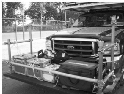
Figure 19.54 Everything has a safety tie on it.
