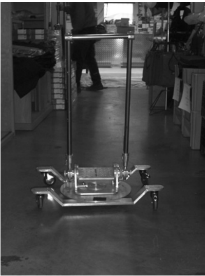
Figure 19.73 Spider rolling camera mount (Modern Studio Equipment).
