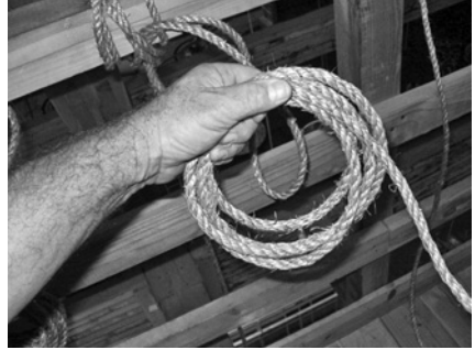
Figure 19.85 Loop through center.
