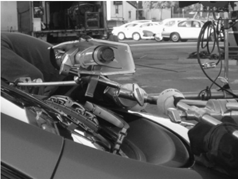
Figure 19.51 Rigging a Kino flow eye light. The tennis balls are used to prevent hitting the glass or paint. Notice the black cloth under straps.
