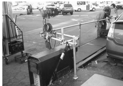
Figure 19.42 Rigging a back light for passenger's head.
