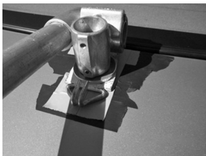
Figure 19.26 Lip clamp (Modern Studio Equipment).
