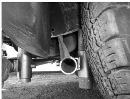
Figure 19.24 Crank-type motorcycle strap through the tube attached to the undercarriage.
