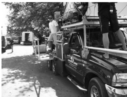
Figure 19.55 Wrong work shoes.
