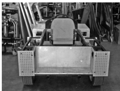
Figure 19.75 Cheese plate-covered “electric” (golf) cart (running/bicycle shots), very quiet (Modern Studio Equipment).
