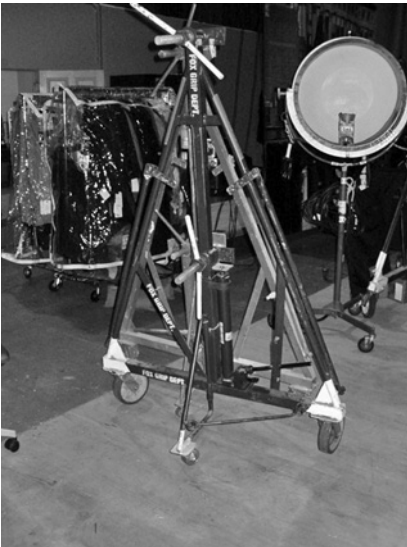
Figure 19.125 Rolling wall jacks with hydraulic lifts.
