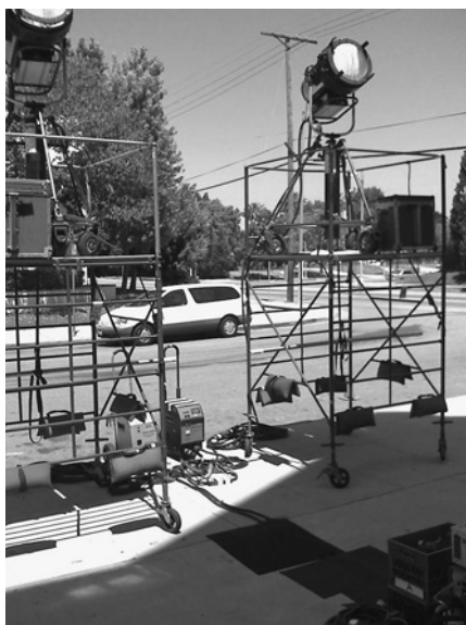
Figure 19.153 How to safety tie down a lamp on a set of parallels.
