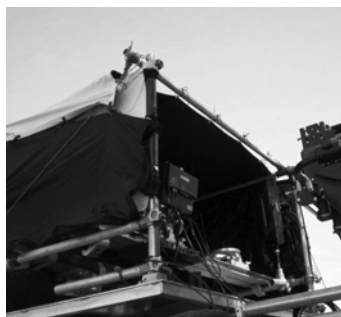
Figure 19.53 Notice sash (rope) tying down corners.
