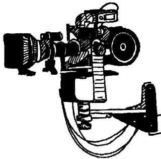
Figure 10.30b Barber Boom Head (top slung).
