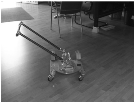
Figure 19.73 Spider rolling camera mount (Modern Studio Equipment).
