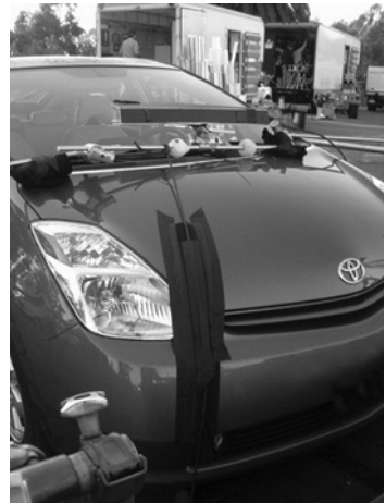
Figure 19.51 Rigging a Kino flow eye light. The tennis balls are used to prevent hitting the glass or paint. Notice the black cloth under straps.
