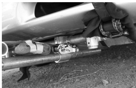
Figure 19.23 I used starter plugs (note the padding under straps).
