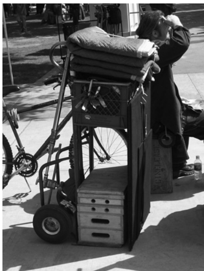
Figure 19.155 High Hat package: 2 each apple boxes, 2 flags, 2 stands, 6 grip clips, 2 6-ft piece of duvatyne, 2 sound blankets, 2 sand bags, dulling spray, streak and tips sprays, 6 wedges. (Complements to Key Grip Jerry Day and his great crew in Local#80).
