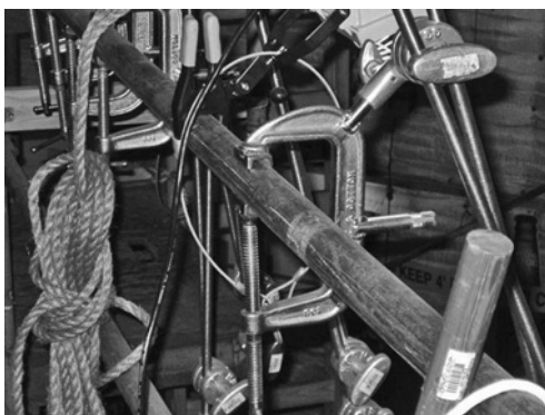
Figure 19.104 Meat axe (made with gobo head).
