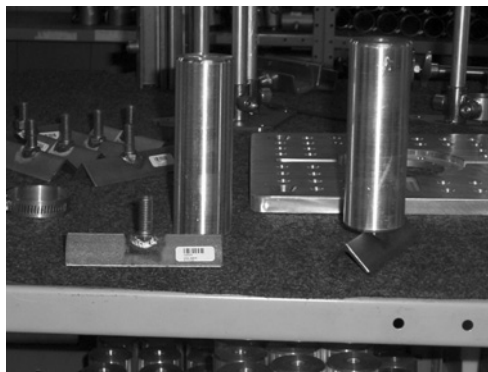
Figure 19.34 Channel (V) with threaded (3/8–16 pitch) threads for “starter plugs.”
