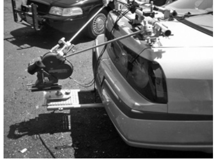
Figure 19.29 Bracing using C-stand arms.
