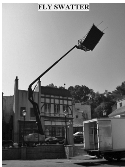
Figure 19.156 Fly swatter with plastic ivy (breaks up the frame edge).
