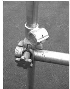
Figure 19.46 Slide the tubes inside the upright tubes. Now install a cross and secure it to the trailer by tying it down.
