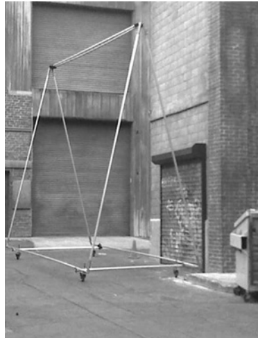
Figure 19.8 Rolling A-frame base built from speed rail, TM corners, 90-degree crosses, and casters/rollers.
