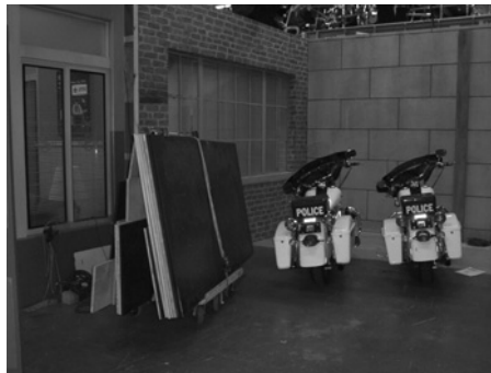
Figure 19.68 Rolling dance floor cart (4 × 8 plywood and 1/4 plastic covers). The wheel in center is larger. This allows tipping up or down to roll over objects such as cable.
