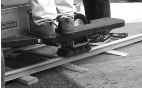
Figure 19.66 Channel wheels used on dolly on track (normal usage).
