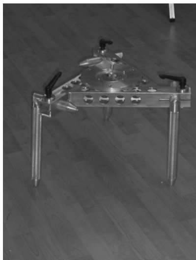
Figure 19.70 Dexter-style spider legs (Modern Studio Equipment).
