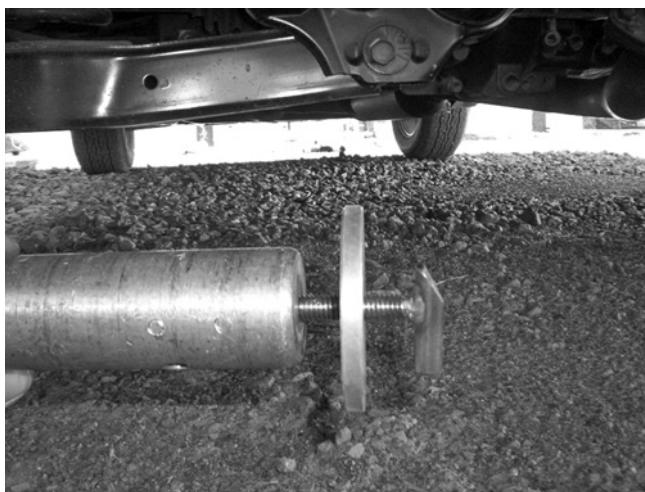
Figure 19.20 What it looks like with the starting "foot," a 3/16 pitch threaded rod that is 3/8-in. in diameter welded to a steel foot—this has worked just fine for many years. From Modern Studio Equipment.
