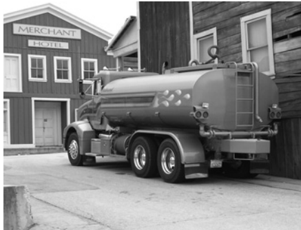
Figure 19.144 Water truck for wet downs.
