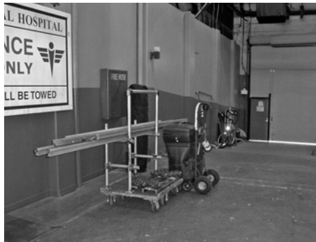
Figure 19.63 Rolling dolly track cart.
