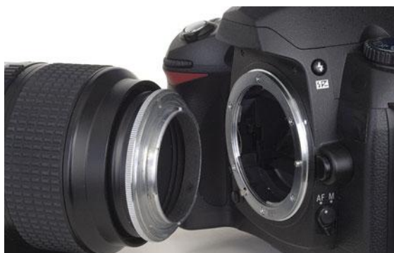
Figure 15.15 A reversing ring lets you mount a lens backwards, which sometimes lets you focus more closely and can improve image quality.
