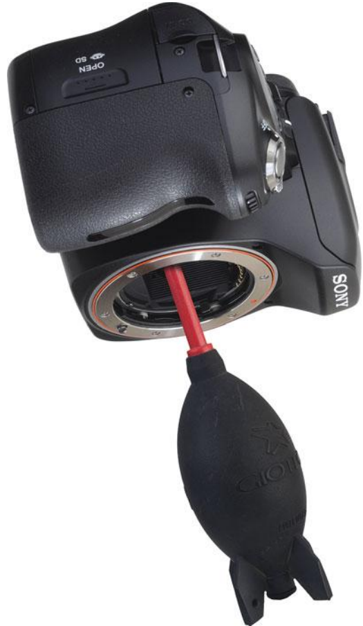
Figure 4.11 A few puffs of air should clean your sensor.
