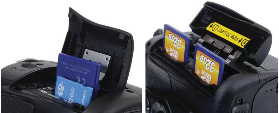
Figure 4.12 Some Sony cameras (left) have two slots: one for Memory Stick Pro cards and one for SD cards, but both can't be used simultaneously. An increasing number of cameras have two slots, and allow you to specify how the card in the second slot is used.
