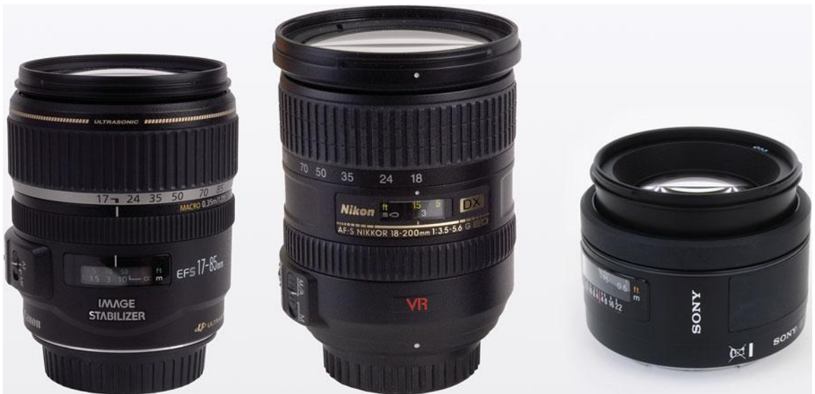
Figure 5.1 Canon's EF-S series (left) and Nikon's DX lenses (middle) can be used only on their digital SLRs with sensors smaller than 24 \times 36 mm. The Sony lens (right) can be used on any Sony or Minolta/Konica Minolta SLR.
