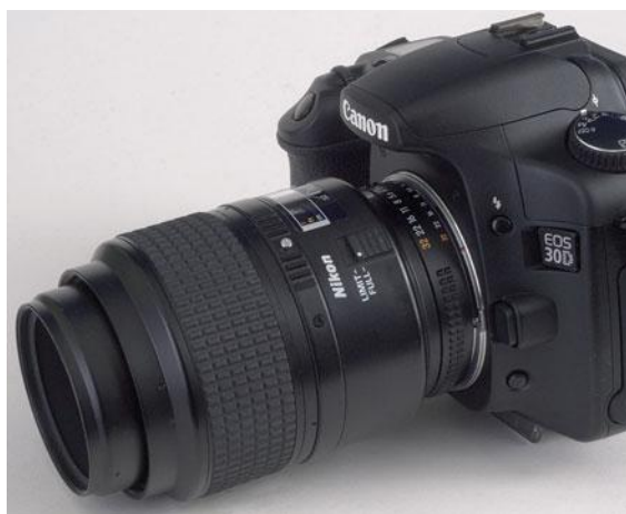
Figure 15.14 If you have or can borrow a Nikon macro lens, you can fit it to your Canon dSLR with an adapter.
