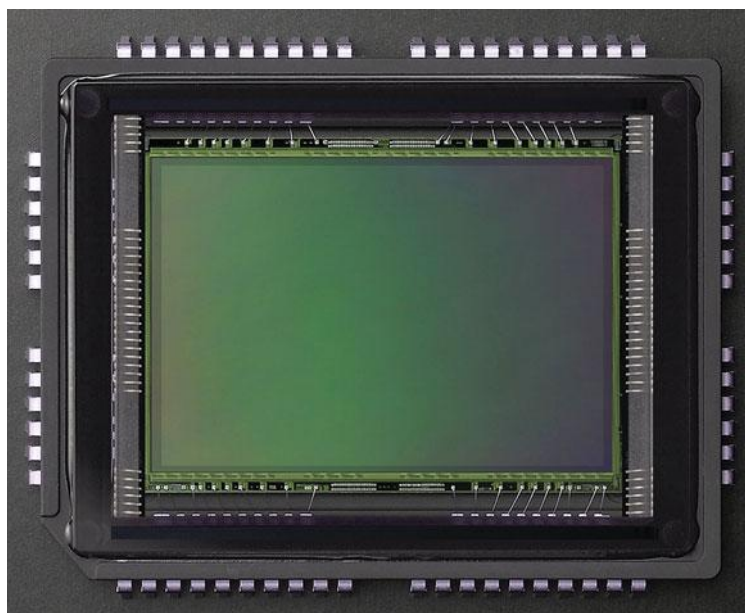
Figure 1.4 A digital SLR sensor looks something like this.
