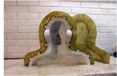
FIGURE 3.9 Front and back halves of a fiberglass matrix mold. Image reproduced by permission of Neill Gorton.
