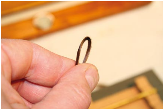
FIGURE 8.26 Pull a small amount of hair from the mats and about 2 inches from the root end of the hair, bend it into a loop called the turnover , and pinch the loop between your thumb and index finger. Photo by the author.
