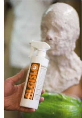
FIGURE 3.27 Algiso® slows the cure of alginate and helps alginate stick to alginate. Photo by Chase Heilman. Image reproduced by permission of the author.
