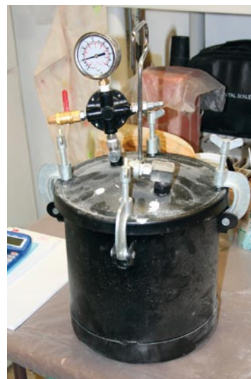
FIGURE 5.25 A 2-gallon pressure/ vacuum chamber from Harbor Freight. Photo by the author.
