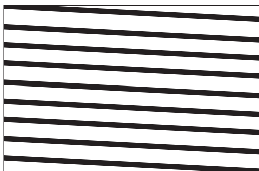
Figure 7.4 Effects of maladjusted timebase controls
