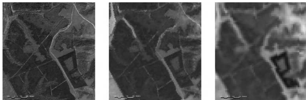
Fig. 4.2. Different resolution of remotely sensed images for the same area. Left: Quick Bird image (pixel of 2.8 m). Centre: SPOT XS (pixel of 10 m). Right: Landsat 7 ETM+ (pixel of 30 m). All images are compositions of RGB 432 in grey-scale palette.
